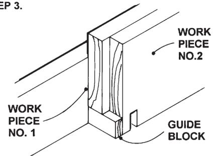
Step 3: Butt the 2<sup>nd</sup> workpiece tightly against the guide block, as shown. Then make a cutting pass to form the notch in both pieces simultaneously.
