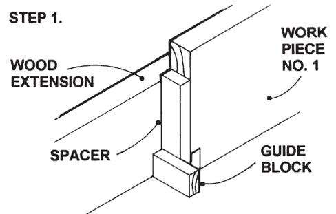
Step 1: Cut a spacer strip with dimensions that equal the groove width and insert it between guide block and 1<sup>st</sup> workpiece. Then, while holding the workpiece firmly, make the first cut.
