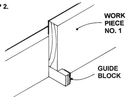
Step 2: Remove the spacer and move the workpiece over until it rests snugly against the spacer block.
