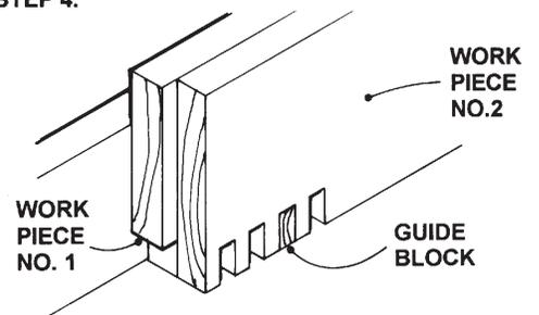
Step 4: Continue making cuts by placing the last notch cut over the guide block to position the boards for the next cut. Note: To ensure boards staying aligned together throughout the cutting process, use small c-clamps, if necessary.
